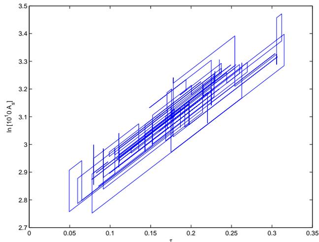
FIG. 4: 2D example sampling fast (vertical) and correlated slow (horizontal) variables.
